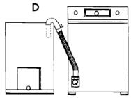
If a longer drain hose is needed, drain hose (Part No. 388423) and hose extension kit (Part No. 285442) are available from authorized parts distributors. If drain hose must be shortened, use hose kit (Part No. 285442)
